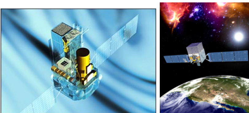
Figure 1.3.1: Space-based gamma-ray telescopes INTEGRAL (detects gamma-rays with energies below 1 MeV) and Fermi (GeV gamma-rays).
